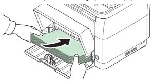
**IMPORTANT** Adjust so that there is no gap between the paper length guide and the paper.
